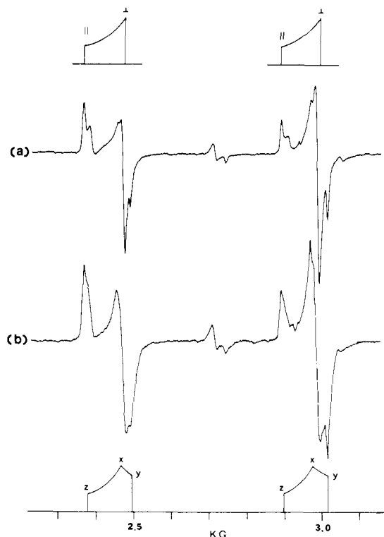
Figure 2. The lower field components ( m_l = +3/2 and +1/2 ) of the B signals observed from (a) the Au/CO(2%)/Ar system and (b) the Au/CO(4%)/Ar system. The absorption patterns of the recognized axially symmetric and orthorhombic systems are indicated.
